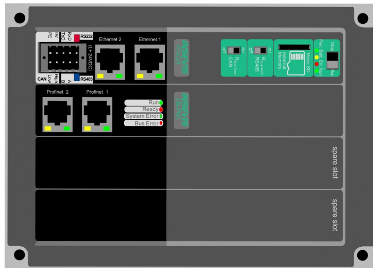
Figure above: View to rear side and connections sides of PC433T-PNC (horizontal use)
