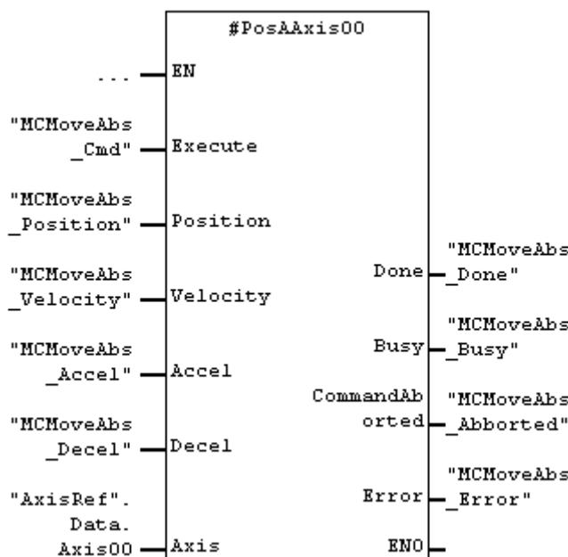
In the STAT-area instanciated MC\_MoveAbsolute\_E2 with the instance name PosAAxis00.
