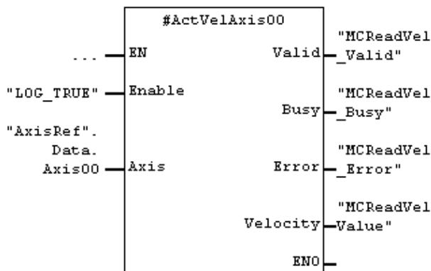
In the STAT-area of a Container-FB instanciated MC\_ReadActualVelocity\_E2 with the instance name ActVelAxis00.
