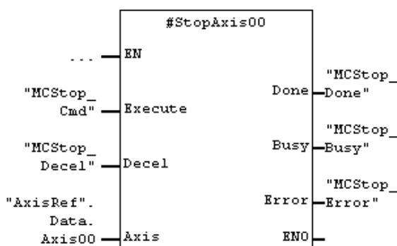
In the STAT-area instanciated MC\_Stop\_E2 with the instance name StopAxis00.
