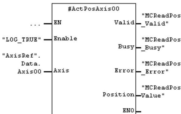
In the STAT-area of a Container-FB instanciated MC\_ReadActualPosition\_E2 with the instance name ActPosAxis00.
